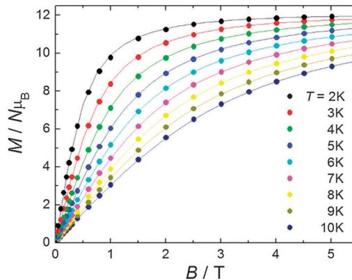
**Fig. 2** (Circles) Experimental isothermal magnetization curves for fields up to *B* = 5 T and taken at several *T*, as labelled. The solid lines are the calculated magnetization curves, see the main text for details.
