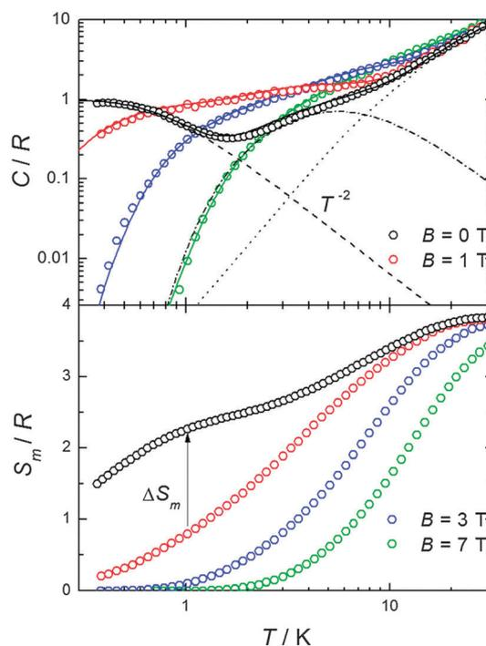
**Fig. 3** Top: temperature dependence of the heat capacity *C* normalized to the gas constant *R* and measured in the presence of several magnetic fields, as labelled. Fit of heat capacity (solid lines) is calculated as explained in the text. Lattice (dotted line) and magnetic (dot-dashed lines, dashed lines) contributions are shown. Bottom: experimental magnetic entropies as obtained from the corresponding *C* data.
