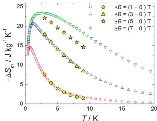
**Fig. 4** Temperature-dependencies of the magnetic entropy change  $\Delta S_m$ , for the indicated applied-field changes  $\Delta B$ , as obtained from heat capacity (empty markers) and magnetization (full markers) measurements.
