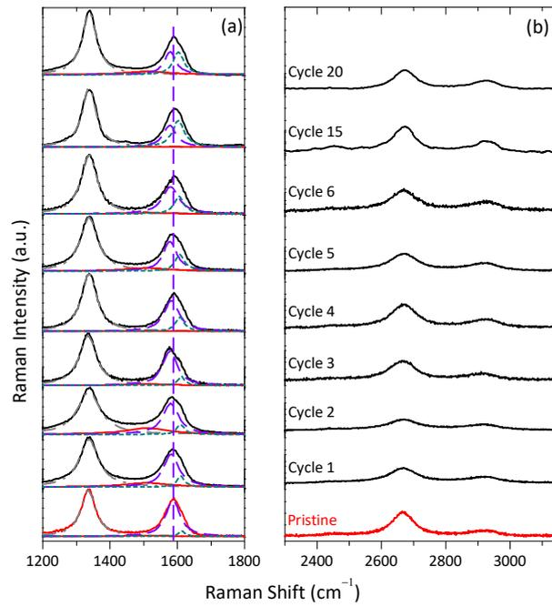
**Fig. 6** Raman spectra of a CNHs sample recovered after different consecutive stress cycles up to *ca.* 2 GPa. Labels indicate the maximum cycle number reached for each sample. The red spectrum at the bottom corresponds to that of the pristine CNHs sample.
