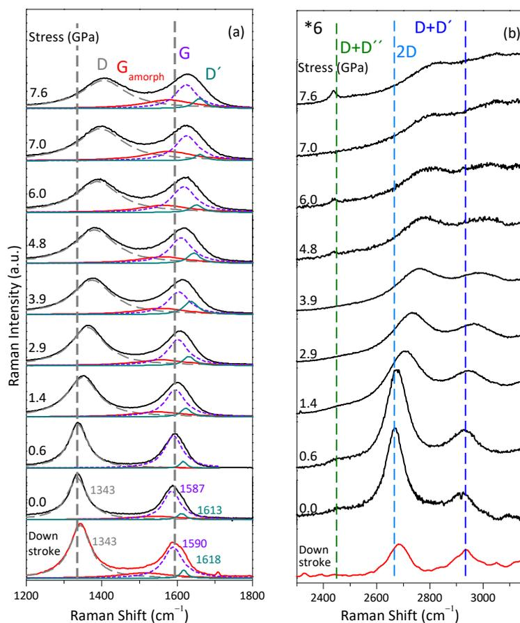
**Fig. 2** Raman spectra of CNHs with increasing stress. (a) Fundamental bands in the spectral range  $1200\text{-}1800\text{ cm}^{-1}$  and (b) combination bands and overtones from  $2300\text{ to }3500\text{ cm}^{-1}$ . In (a) the Lorentzian functions representing the most relevant bands are plotted in different colors.
