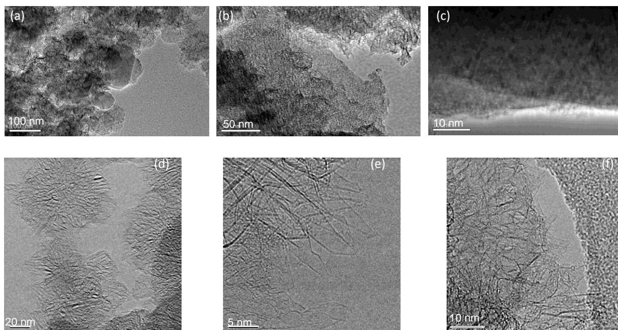
**Fig. 5** TEM images at different magnifications of the CNHs sample recovered after a 8 GPa stress cycle, in two different regions, A (a-c) and B (d-f), with graphite-like amorphous carbon and broken dahlias morphologies, respectively.
