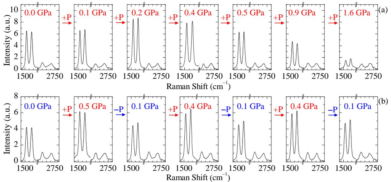
FIG. 1. Evolution of Raman spectra of  $^{13}\text{C}/^{12}\text{C}$  tBLG (a) with compression up to 1.6 GPa, and (b) with stress cycling of  $\pm 0.4$  GPa, approximately. Laser excitation energy of 488.0 nm.
