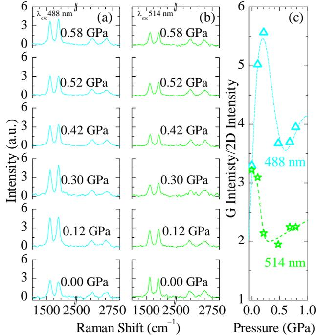
FIG. 3. Evolution of the Raman spectra of <sup>13</sup>C/<sup>12</sup>C tBLG with compression up to 0.6 GPa. The same tBLG grain is measured with (a) 488.0 nm and (b) 514.5 nm excitation energy. (c) Intensity ratio G/2D as a function of increasing stress.
