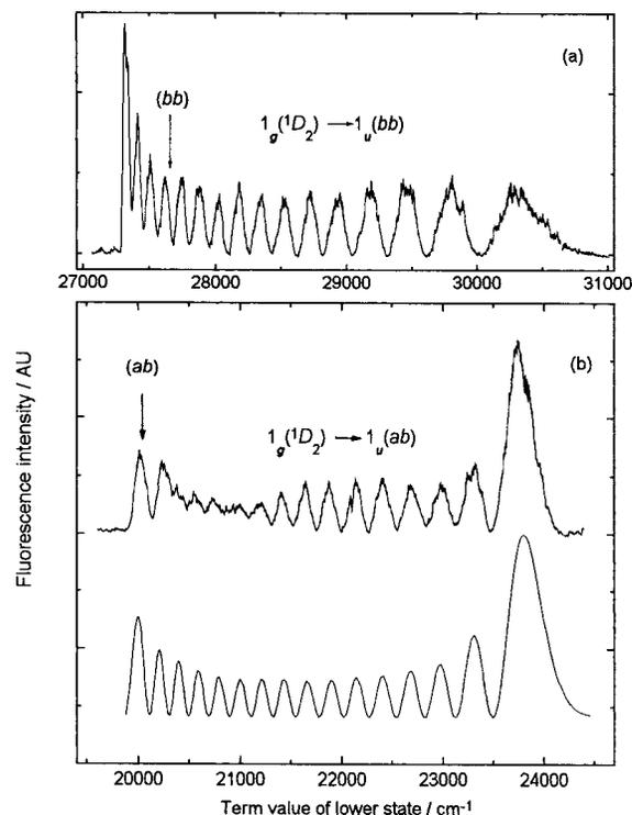
FIG. 2. Emission from  $v=15, J=31$  of the  $1_g(^1D_2)$  state, (a) to the only  $1_u$  state that correlates with the  $(bb)$  dissociation limit and (b) to one or both of the  $1_u$  states that correlate with the  $(ab)$  dissociation limit. A simulation of the fluorescence to the more deeply bound of the two lower states is shown. The term value, relative to  $v=0, J=0$  of the  $X0_g^+(aa)$  state, of the level on which the emission terminates, is shown on the  $x$  axis.
