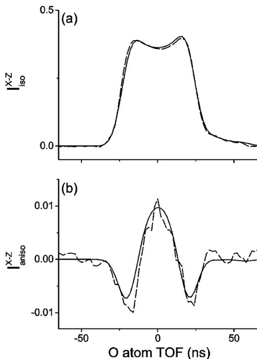
FIG. 6. Isotropic and anisotropic TOF profiles of O(<sup>3</sup>P<sub>2</sub>) products at photolysis wavelength 223.543 nm: (a)  $\mathbf{I}_{\text{iso}}^{X-Z}$ , (b)  $\mathbf{I}_{\text{aniso}}^{X-Z}$ . Experimental data are shown as dashed lines, fitted data are solid lines.
