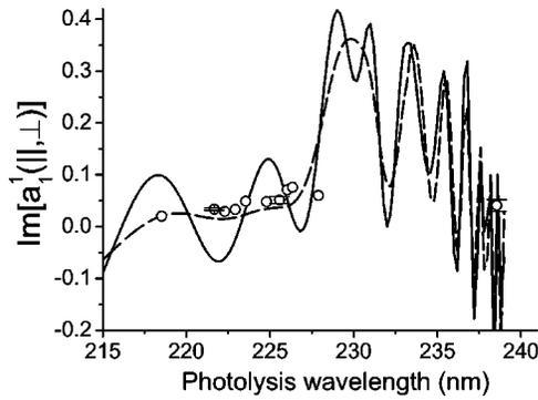
FIG. 7. Molecule frame orientation parameter  $\text{Im}[\mathbf{a}_1^{(1)}(\parallel, \perp)]$  for  $\text{O}(^3P_2)$  atoms vs photolysis wavelength. Circles are experimental points. The solid line is the semiclassical simulation obtained using potential energy curves of VG [see Eq. (15) (Ref. 8)]. The dashed line incorporates a reduction in the term involving the  $c0$  state. See text for details.
