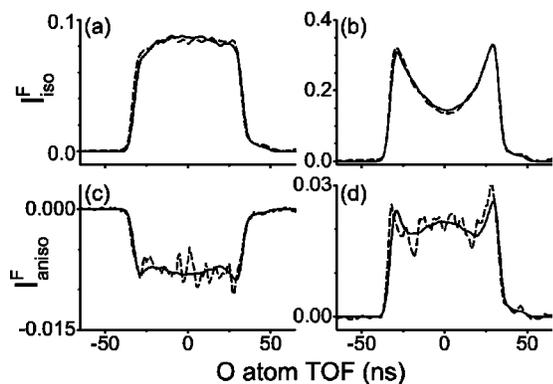
FIG. 1. Isotropic and anisotropic TOF profiles of O(<sup>3</sup>P<sub>2</sub>) products at photolysis wavelength 222 nm: (a)  $I_{\text{iso}}^X$ , (b)  $I_{\text{iso}}^Z$ , (c)  $I_{\text{aniso}}^X$ , (d)  $I_{\text{aniso}}^Z$ . Experimental data are shown as dashed lines, fitted data are solid lines.
