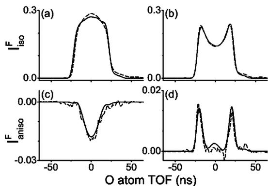
FIG. 2. Isotropic and anisotropic TOF profiles of O(<sup>3</sup>P<sub>2</sub>) products at photolysis wavelength 237 nm: (a)  $I_{\text{iso}}^X$ , (b)  $I_{\text{iso}}^Z$ , (c)  $I_{\text{aniso}}^X$ , (d)  $I_{\text{aniso}}^Z$ . Experimental data are shown as dashed lines, fitted data are solid lines.
