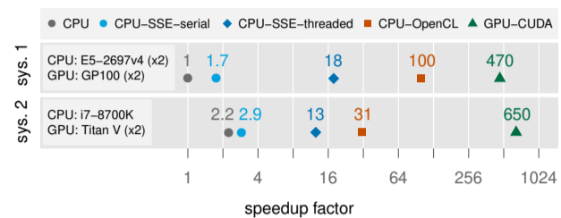
FIGURE 3. Relative performance gains (fold-speedup) on two systems for analysis with BEAST v1.10.5 and BEAGLE v3.1.2 for an unpartitioned codon analysis of the previously-described dengue virus data set (see PERFORMANCE EVALUATION), comprising 3,330 codons. For the BEAGLE GPU implementation, this data set requires 21.5 GB of memory and thus we scale computation by pattern block across two library instances, each running on a separate GPU. Benchmarks are for 10,000 iterations, and the single-threaded, non-vectorized, version of BEAGLE CPU running on system 1 is used as a reference.
