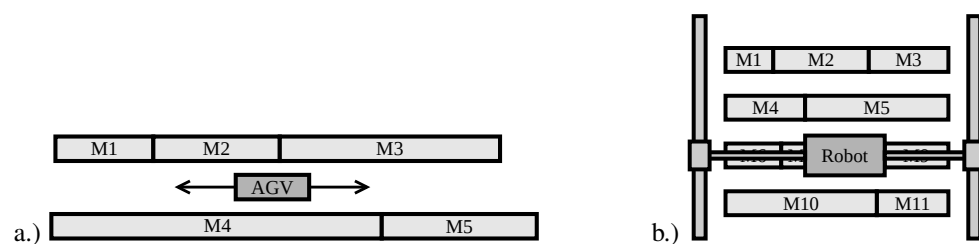
Figure 2: In a.) an AGV transports parts between the machines that are located on both sides of a linear path of travel. In b.) a gantry robot is used when the space is limited.
