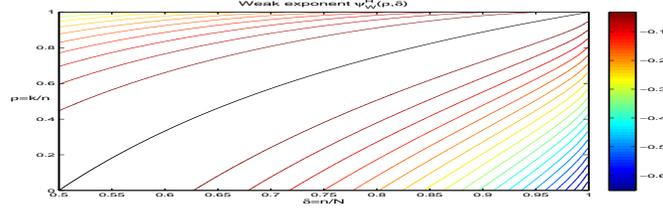
FIGURE 2.1. Exponent for the weak phase transition,  $\psi_W^{\mathbb{R}^+}(\rho, \delta)$ , (2.10), which has its zero level curve at  $\rho_W(\delta; \mathbb{R}_+)$ , equation (1.3). The projected hypercube has the same weak phase transition and exponent  $\psi_W^I \equiv \psi_W^{\mathbb{R}^+}$ .
