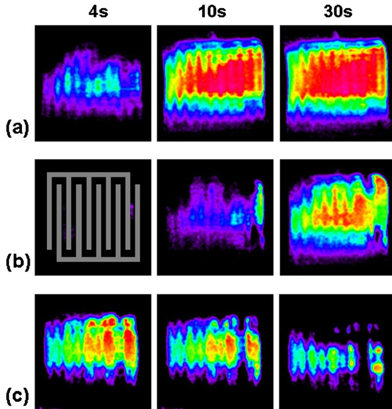
FIG. 5. Color coded TIRF images extracted from rRNA DEP movies at 4, 10, and 30 s after the onset of a  $4 V_{pp}$  ac field set at: (a) 100 kHz, (b) 3 MHz, and (c) 50 MHz measured after positive DEP at 100 kHz. Image processing included background subtraction and Gaussian smoothing. An outline of the electrode is superimposed on the first image of the 3 MHz series (enhanced online).
