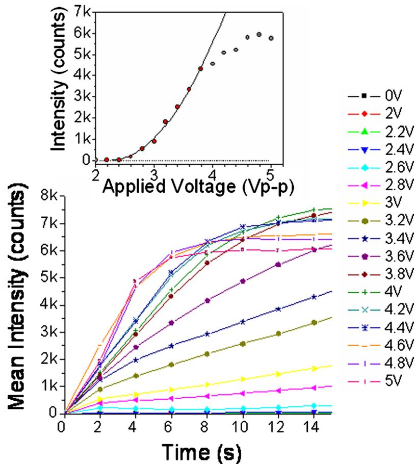
FIG. 4. DEP voltage dependence measured at 1 MHz. Intensity time traces obtained from 0 to 5  $V_{p-p}$ . In inset is shown the DEP voltage dependence plotted at 6 s after the onset of DEP, along with the quadratic function  $F$  (line) given by the equation  $F = A(V - V_{\min})^2$  with  $A = 1774$  and  $V_{\min} = 2.23$ . The quadratic dependence of the DEP is observed between  $V_{p-p} = 2.2$  and  $3.8$  V.
