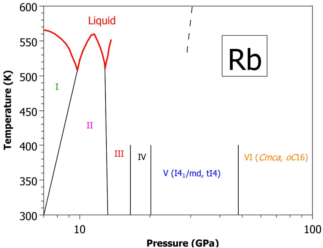
**Figure 1.** (Color on line) High-pressure phase diagram of Rb<sup>13,14,16,15,17,18,20,3</sup>. The dashed line is a hypothetical phase boundary passing through the only single melting point observed along an isotherm decompression at 573 K. The high temperature extensions of the solid-solid phase transitions are also hypothetical, as these phase transitions have only been investigated at room temperature.
