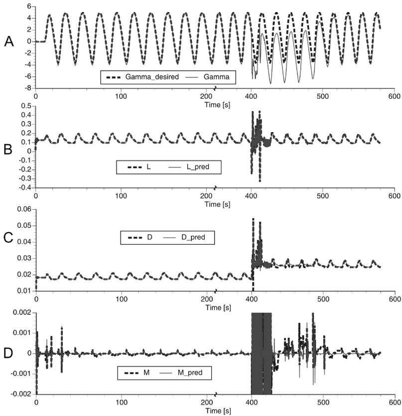
Figure 8: LWPR learning results for adaptive learning control on a simulated autonomous airplane. (A) Tracking of flight angle:  $\gamma$ . (B) Approximation of lift force:  $D$ . (C) Approximation of drag force:  $L$ . (D) Approximation of pitch moment:  $M$ . At 400 seconds into the flight, a failure is simulated that locks one control surface to a 17 degree angle. Note that for clarity of presentation, an axis break was inserted after 200 seconds.
