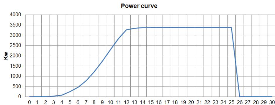
**Figure 2.** Wind turbine Power curve as adapted from [34].
