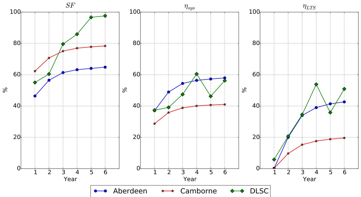
Figure 7: Technical performance metrics for the two UK locations and the original DLSC: Solar Fraction (SF), System Efficiency ( $\eta_{sys}$ ), and Long Term Storage Efficiency ( $\eta_{LTS}$ ).
