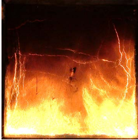
(i) Crack initiation, 0.00 s
