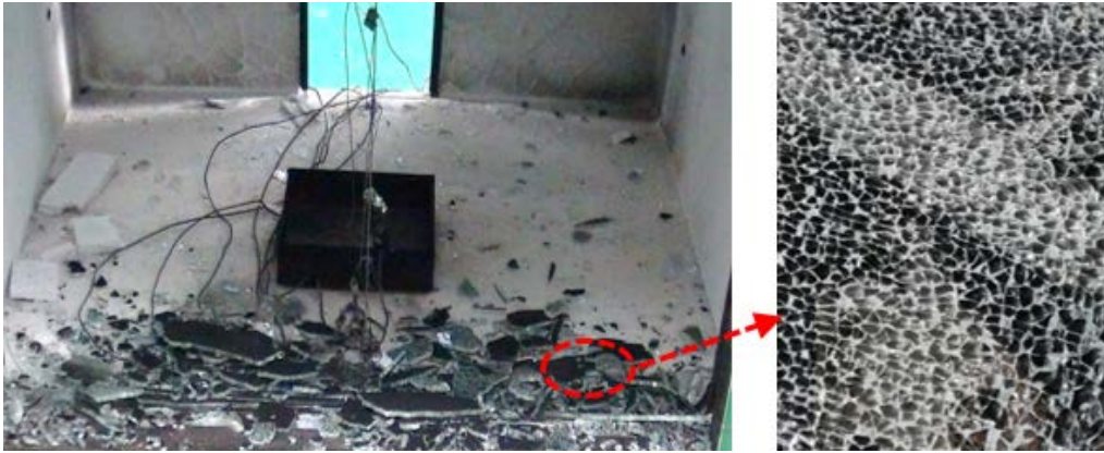
(b) The post crack path of tempered glazing
