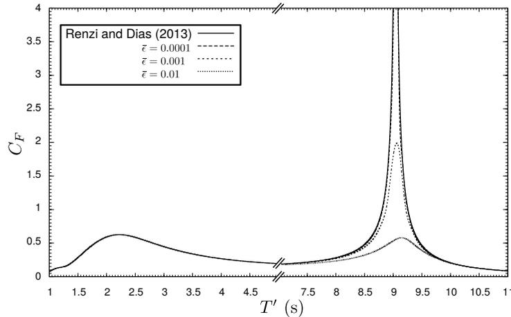
Figure 2: The influence of dissipation on the capture factor of an OWSC with spike at the resonant wave period at  $T' \approx 9$  s.
