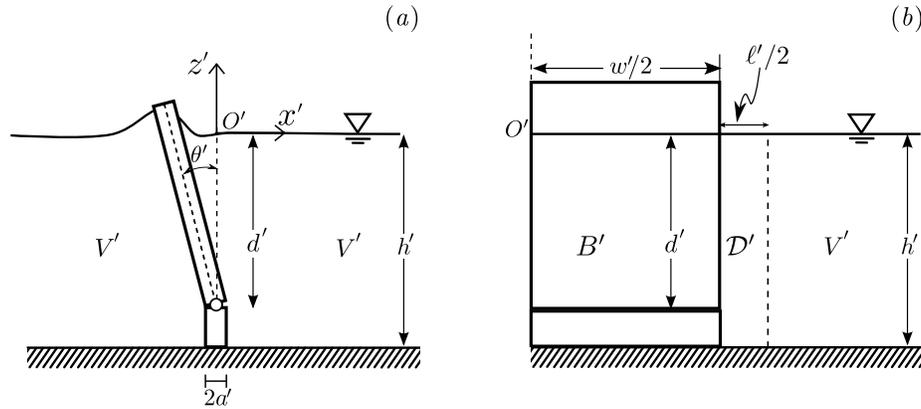
Figure 1: The geometry of the surface-piercing OWSC with dissipative surface  $\mathcal{D}'$ : (a) section (b) front view.
