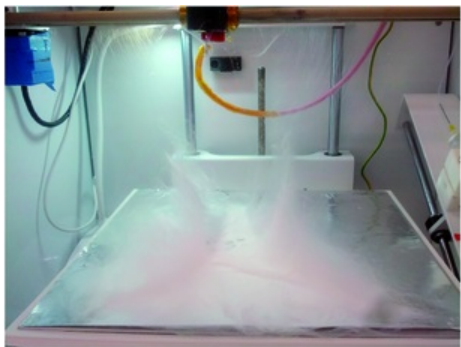
Fig. 10 At a working distance of 10 cm, the electrospun fibers were attracted to the rubber belt of the moving nozzle. 15.0 wt% PS in 1 : 1 DMF/THF was electrospun at 20 kV, a flow rate of 5.0 mL h -1 , at a nozzle moving speed of 12.0 mm s -1 , at ambient conditions.
