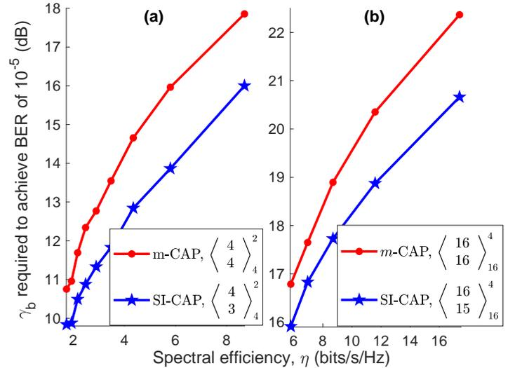
Fig. 5. Comparison of the  $\gamma_b$  required by SI-CAP and *m*-CAP to achieve BER of  $10^{-5}$  in a bandwidth-limited VLC system modelled using a first-order low pass filter with  $\mathcal{T} = 2$  and 4 bpcu.
