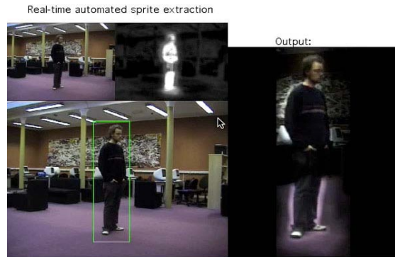
Figure 6: Automatic extraction of video sprites from real life
