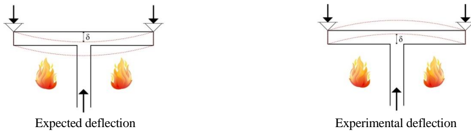
Figure 2 Conceptual arrangement for testing heated flat plate beam-column connections. (a) Expected deflection response under heating and (b) Deflection response observed in Smith's tests [4–6].
