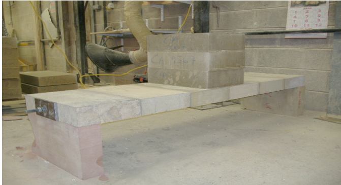
Figure 1 Initial post-tensioned stone panel, 100 millimetres deep, with an effective span of 1.76 metres. Load is applied using stone blocks.
