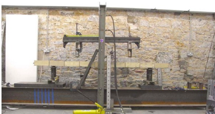
Figure 6 Test rig and loading arrangement for stone panels
