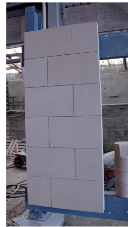
Figure 4 Prototype post-tensioned stone panel erected on test rig
