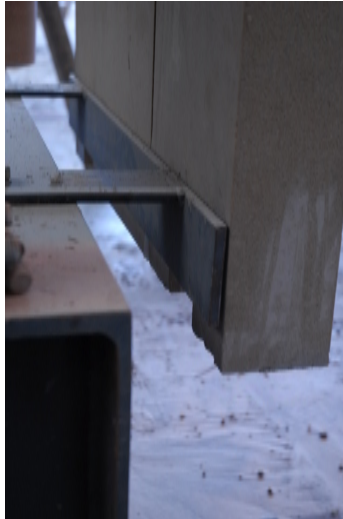
Figure 5 Combined connection and post-tensioning anchorage
