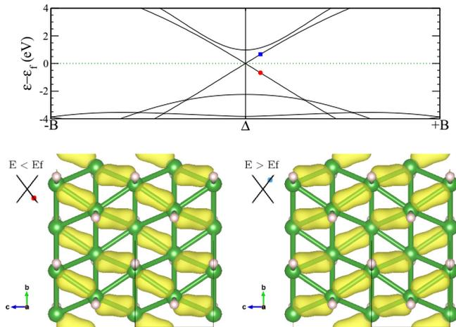
FIG. 3. Top: Detail of the band structure of 2D borane, passing through  $\mathbf{k}_d$  and perpendicular to  $\Gamma Y$ . Bottom: Charge densities associated with the highlighted  $k$  points in the band structure.
