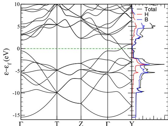
FIG. 2. Band structure and density of states (DOS) of the single-layer 2D borane. The DOS has been computed using OptaDOS [50].
