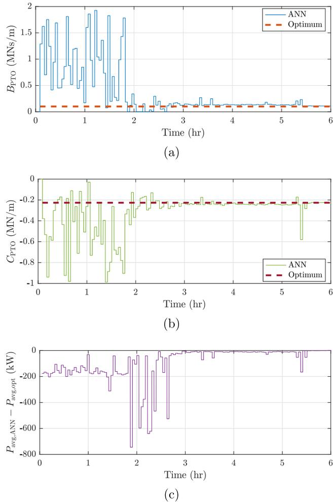
**Fig. 7.** PTO damping (a) and stiffness (b) coefficients obtained from the ANN-based control as compared with the optimal value in regular waves with  $H_s = 2$  m and  $T_e = 8$  s. (c) shows the difference in the corresponding mean generated power.
