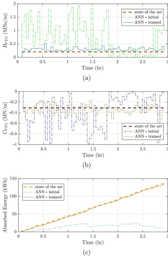
**Fig. 8.** PTO damping (a) and stiffness (b) coefficients adopted by the ANN-based control at the start and after 54-h of training in the wave conditions shown in Table 1 in irregular waves with  $H_s = 2$  m and  $T_e = 8$  s. Additionally, (a) and (b) display the results of state-of-the-art reactive control. The corresponding curves for the absorbed energy are plotted in (c).
