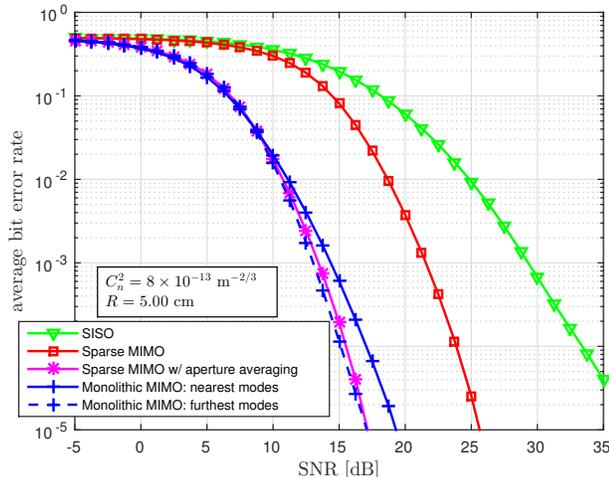
Fig. 9. The average BER versus SNR  $\gamma$  when  $C_n^2 = 8 \times 10^{-13} \text{ m}^{-2/3}$  and  $R = 5.00 \text{ cm}$ . For monolithic MIMO, the nearest modes refer to the mode set  $\{-1, 0, +1\}$  and the furthest modes refer to the mode set  $\{-8, 0, +8\}$ .
