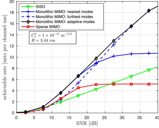
Fig. 4. The average achievable rate for different schemes versus SNR ( $P/\sigma$ ) when  $C_n^2 = 1 \times 10^{-15} \text{ m}^{-2/3}$  and  $R = 3.44 \text{ cm}$ . For monolithic system, the nearest modes refer to the mode set  $\{-1, 0, +1\}$  and the furthest modes refer to the mode set  $\{-3, 0, +3\}$ .
