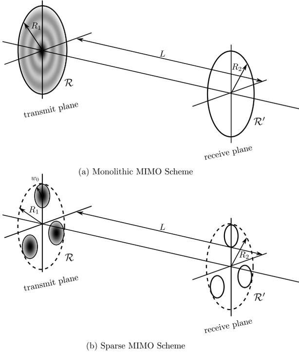
Fig. 2. A Schematic diagram of a MIMO FSO system whether implemented based on a) monolithic or b) sparse apertures. The input beam pattern  $\xi(\mathbf{r})$  can be properly defined over the transmit aperture  $\mathcal{R}$  to describe either design.
