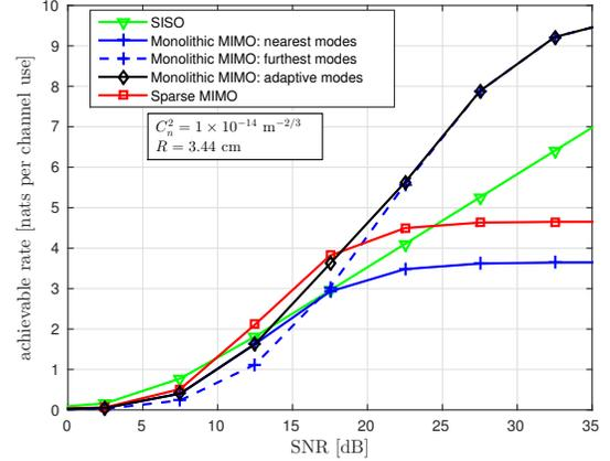
Fig. 6. The average achievable rate for different schemes versus SNR ( $P/\sigma$ ) when  $C_n^2 = 1 \times 10^{-14} \text{ m}^{-2/3}$  and  $R = 3.44 \text{ cm}$ . For monolithic system, the nearest modes refer to the mode set  $\{-1, 0, +1\}$  and the furthest modes refer to the mode set  $\{-3, 0, +3\}$ .
