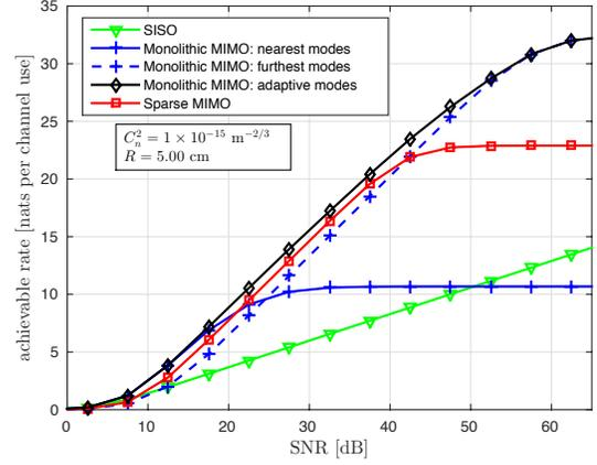
Fig. 5. The average achievable rate for different schemes versus SNR ( $P/\sigma$ ) when  $C_n^2 = 1 \times 10^{-15} \text{ m}^{-2/3}$  and  $R = 5 \text{ cm}$ . For monolithic system, the nearest modes refer to the mode set  $\{-1, 0, +1\}$  and the furthest modes refer to mode set  $\{-8, 0, +8\}$ .
