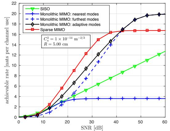
Fig. 7. The average achievable rate for different schemes versus SNR ( $P/\sigma$ ) when  $C_n^2 = 1 \times 10^{-14} \text{ m}^{-2/3}$  and  $R = 5 \text{ cm}$ . For monolithic system, the nearest modes refer to the mode set  $\{-1, 0, +1\}$  and the furthest modes refer to the mode set  $\{-8, 0, +8\}$ .
