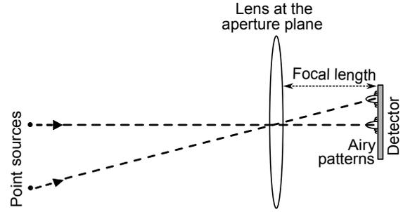
Fig. 1. The Airy pattern images of two beams emitted from distant separated sources are generated by a lens located at the aperture plane of a FSO receiver. The spatial orthogonality of the Airy patterns is demonstrated on the detector area which is positioned at the focal plane of the aperture lens. Note that the size of the detector and Airy patterns ( $\mu\text{m}$  range) are much smaller than the lens (cm range) but they are illustrated in comparable scale for presentation.
