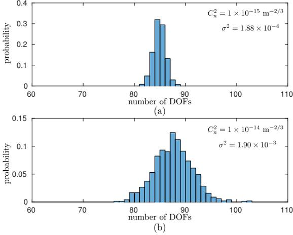
Fig. 3. The histogram of  $D_f$  representing the randomness in the available DoFs of the FSO channel with  $L = 1$  km,  $\lambda = 850$  nm and  $R_1 = R_2 = 5$  cm in different turbulence conditions: (a)  $C_n^2 = 1 \times 10^{-15} \text{ m}^{-2/3}$ , and (b)  $C_n^2 = 1 \times 10^{-14} \text{ m}^{-2/3}$ .
