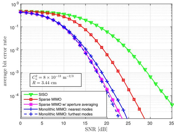
Fig. 8. The average BER versus SNR  $\gamma$  when  $C_n^2 = 8 \times 10^{-13} \text{ m}^{-2/3}$  and  $R = 3.44 \text{ cm}$ . For monolithic MIMO, the nearest modes refer to the mode set  $\{-1, 0, +1\}$  and the furthest modes refer to the mode set  $\{-3, 0, +3\}$ .
