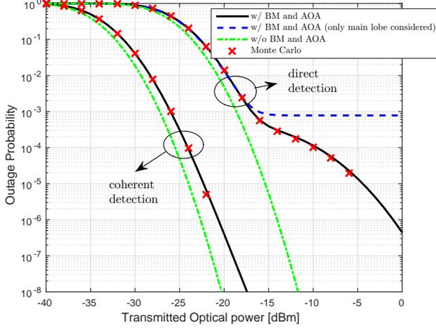
Fig. 6. Outage probability vs. transmitted optical power for FSO receiver in the presence of transceiver vibrations,  $D = 150$  (BM: beam misalignment). Perfect AOA tracking system is employed for coherent detection.
