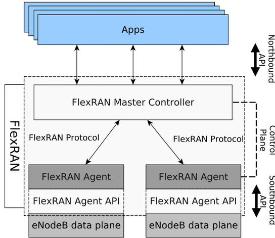
**Figure 1: High-level schematic of the FlexRAN platform.**
