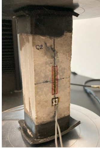
Figure 3: Fibre-cement compressive coupon, wrapped with UD CFRP ribbon
