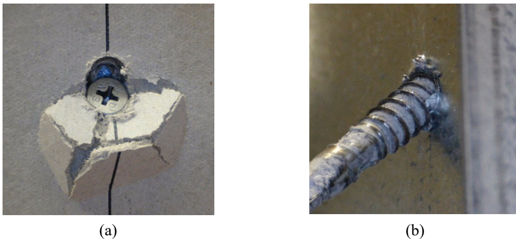
Figure 10: Failure modes - (a) bearing failure and cracking on the board, (b) fastener tilting on the inside of the CFS channel for a wingtip specimen
