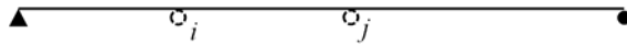
(a) Simply supported beam with an assumed “perturbed” boundary condition with added pins at “i” and “j”
