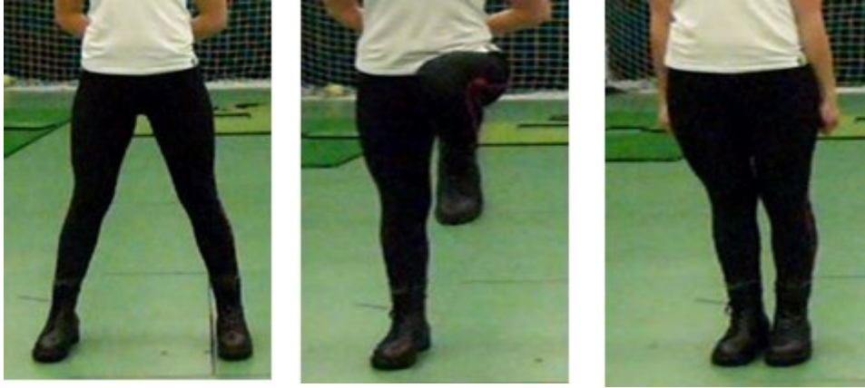
Figure 2. Illustrates a typical SaA British Army foot-drill whilst wearing the CB. From left to right, the SaA is performed from the SaE position. On command, the participant flexes at the hip to 90° followed by an exaggerated stamping of the foot onto the surface of the force plate, landing with the knee in an extended position.
