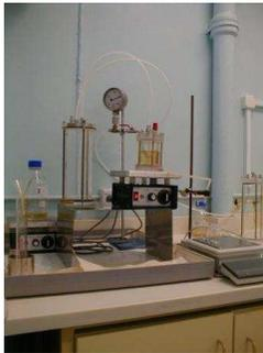
Figur 1 The filtration setup
