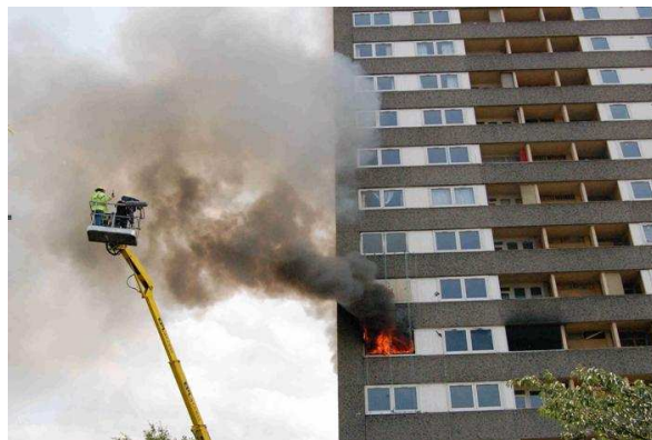
Figure 1: Dalmarnock fire test one seen from outside 18.5 min into the fire
