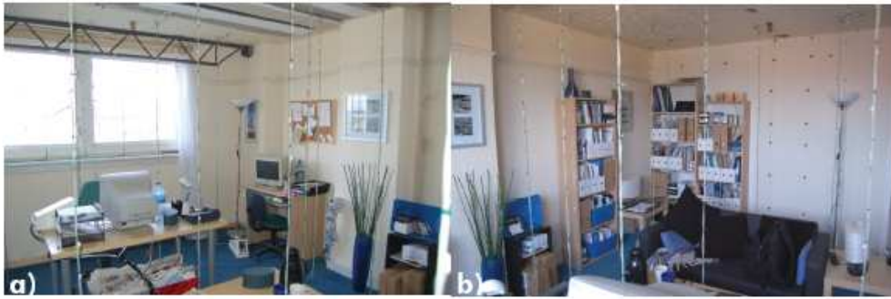
Figure 3: Fuel distribution in compartment fire test
