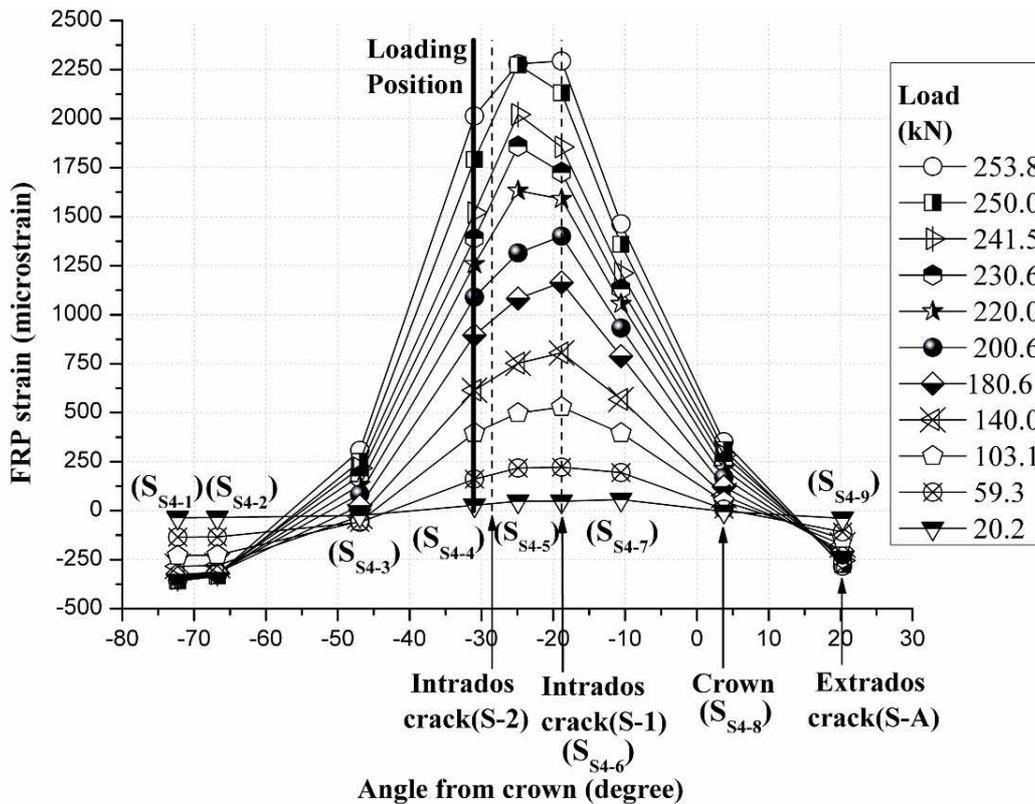
Figure 11. CFRP strain profiles for strain gauges on plate P<sub>s4</sub>
