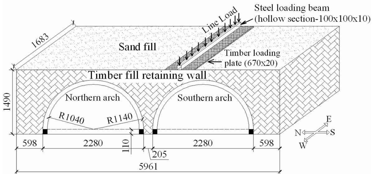
Figure 1. Overview of the arch bridge model (mm)
