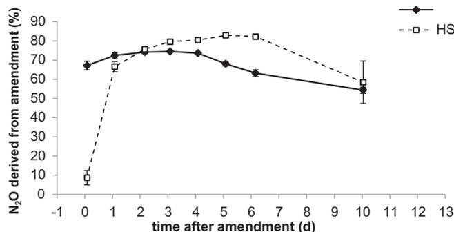
Fig. 3. Portion of N<sub>2</sub>O derived from <sup>15</sup>N enriched amendment in percent of total emitted N<sub>2</sub>O. Error bars are standard error (n = 4).
