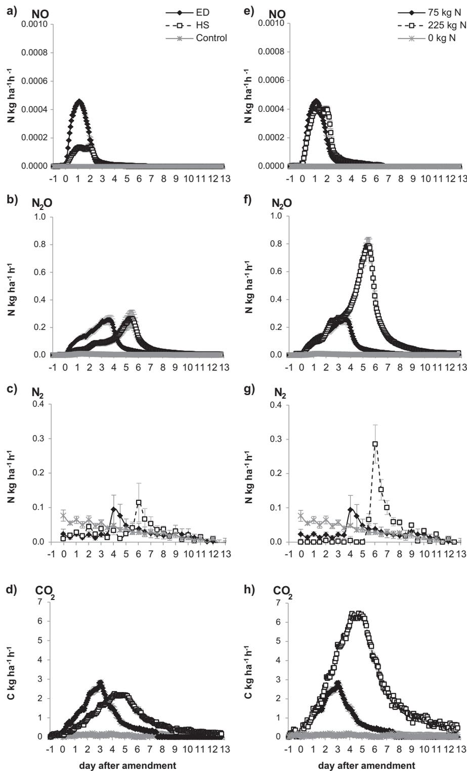
Fig. 2. Average fluxes of NO, N<sub>2</sub>O, N<sub>2</sub> and CO<sub>2</sub> for the different treatments (n = 4). The left side (a–d) shows the gaseous emissions measured per vessel; the right side (e–h) shows emissions based on the concentration of the amendment applied to one core. (1 kg ha<sup>-1</sup> h<sup>-1</sup> = 1.74 × 10<sup>-5</sup> mg cm<sup>-2</sup> h<sup>-1</sup>).
