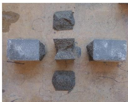
Figure 2: Failure mode of a 15% white ceramic at 29 days (after compressive testing)
