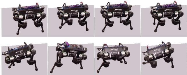
Fig. 13. Comparison between the nullspace and Schur-complement factorizations during a dynamic trotting gait with the ANYmal robot. The Schur-complement factorization is more expensive to compute, and our MPC cannot run at 50 Hz. These delays in the control loop produced instability in the trotting gait (bottom). Instead, the nullspace factorization allowed the MPC to run at 50 Hz and generated a stable trotting gait (top).
