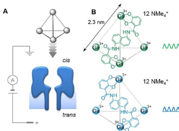
**Figure 1.** (A) Experimental setup in which tetrahedral coordination cages were driven towards the *cis*-opening of a single  $\alpha$ -haemolysin ( $\alpha$ -HL) nanopore inserted in a lipid bilayer under an applied transmembrane potential. (B)  $\Lambda\Lambda\Lambda\Lambda$  (green) and  $\Delta\Delta\Delta\Delta$  (blue) homochiral forms of the Ga(III) cage used in this study. Each grey edge indicates the position of a bridging ligand molecule.
