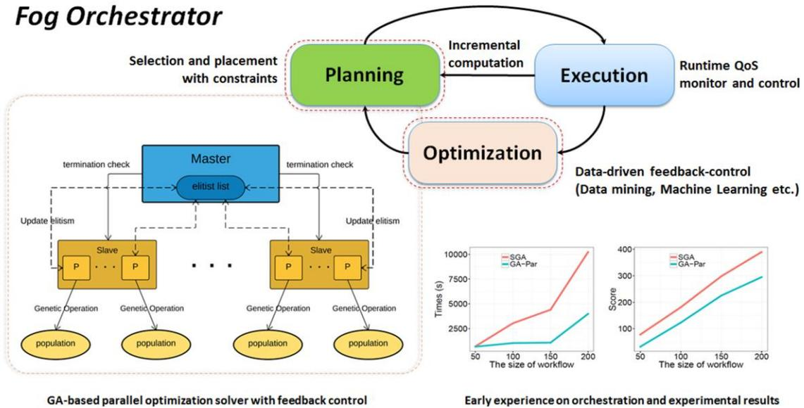
Figure 1: Main functional elements in our Fog Orchestrator: *planning* is responsible for selection and placement, runtime monitoring and control during *execution*, and data-driven decision *optimization*. We propose a parallel GA solver to accelerate the handling of optimization issues raised in the planning and optimization phase. Initial results demonstrate the proposed approach can outperform a standalone genetic algorithm in terms of both time and quality aspects.
