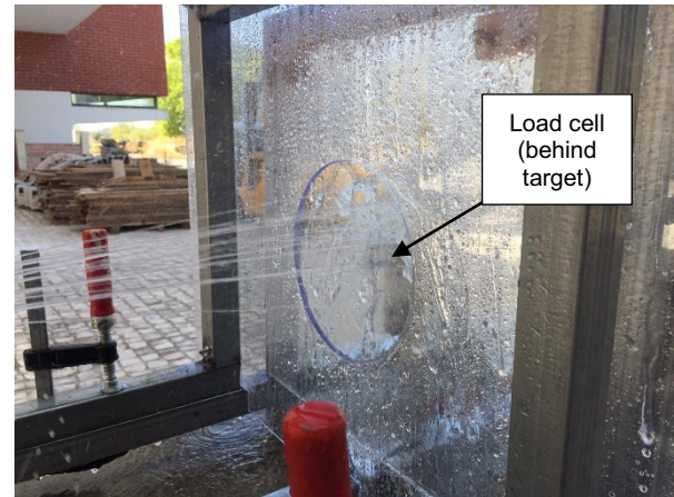
Fig. 3. View of the guard plate (150 mm diameter) in front of the instrumented target panel.
