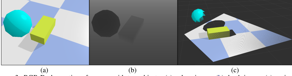
Figure 3: RGB-D observation of a scene with two objects: (a) colour image, (b) depth image, (c) projected colour point cloud in RViz.
