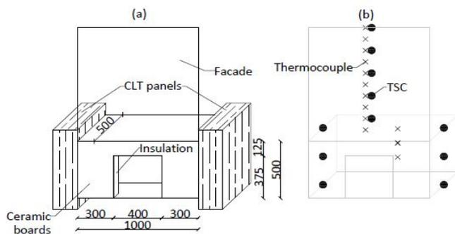
Figure 2 Experimental setup and instrumentation.
