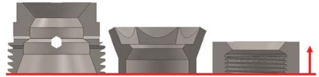
FIG. 6. The final printing sequences of the cell components. The red line is the base-line of the printing process, and the red arrow is the direction of the printing process.
