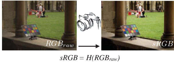
Figure 2: Color correction (mapping raw to display sRGB ) is an homography problem. This figure is also a color chart example which was used for our color correction evaluation.
