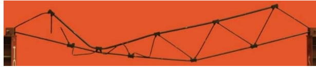
Fig. 14. Truss-RJ collapsed due to the removal of DM2
