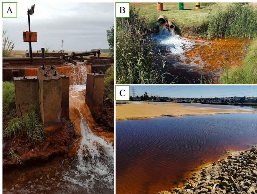
Fig. 1. AMD from underground shafts in Witwatersrand basin, South Africa. In (A) and (B) the effluent is initially colourless with the yellow-boys being visible, and in (C) after oxidation by atmospheric air the effluent gradually turns red.
