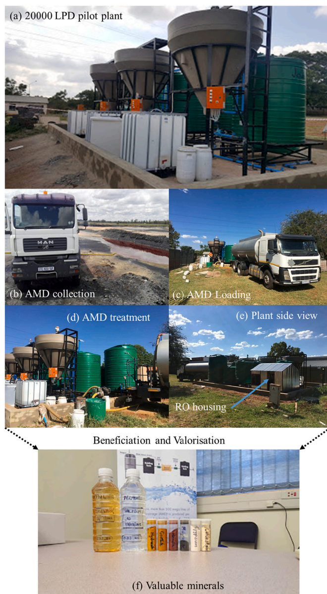
Fig. 7. The MASRO(E) pilot plant at the CSIR, South Africa along with the recovered minerals (photos courtesy of Vhangwele Masindi, Muhammad S Osman, and Rhulani Shingwenyana).
