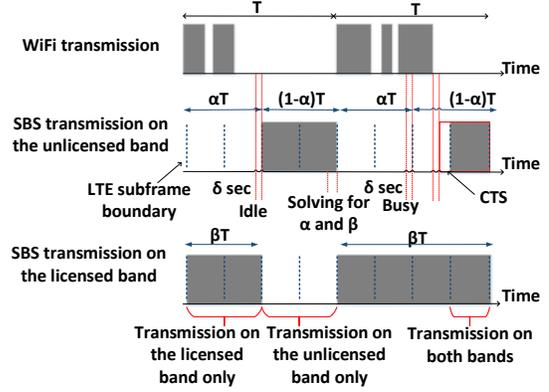
**Figure 2: Illustration of the proposed SBS transmission mechanism on the licensed and unlicensed bands. The two possible states upon sensing the unlicensed channel (idle and busy) are demonstrated. SBS will remain in a sensing state when it encounters a busy channel. The three states of SBS (i.e., transmission on the licensed, unlicensed and both bands) are also shown.**
