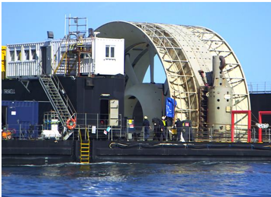
Fig. 1. OpenHydro's 16m Diameter Tidal Device
