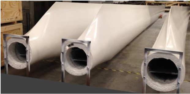
Fig. 3. 13m wind turbine blades made using epoxy powder
