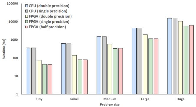
Figure 5: Runtime performance for FPGA kernels and CPU
