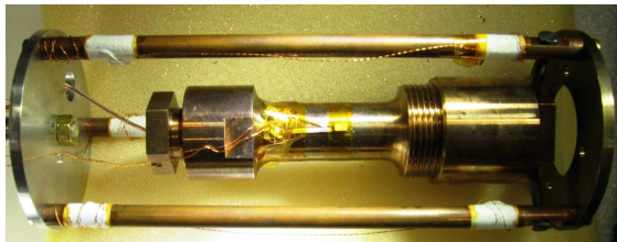
FIG. 4. Loaded cell fixed to the cryostat holder.
