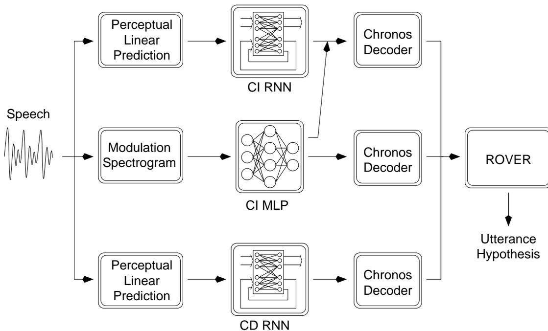
Figure 8: Schematic of the SPRACH Hub-4E Transcription System.
