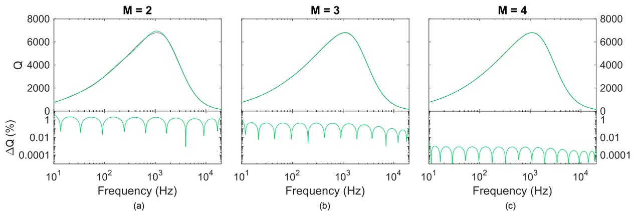
Figure 2:  $Q_{th}(\omega)$  (black line), superposed with optimised approximations to various orders (green line), and associated error  $\Delta Q = \left| \frac{Q_{th} - Q}{Q} \right|$  (%). (a)  $M=2$ ; (b)  $M=3$ ; (c)  $M=4$ .
