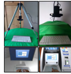
Figure 4: For each setup, we had a physical keyboard, a greenscreen, and a camera to blend the keyboard and users' hands into virtuality, similar to McGill et al. [55] and Oculus' Passthrough API [23].
