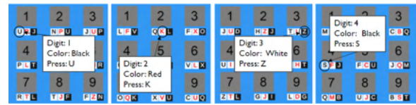
Figure 2: Exemplary ColorPIN [20] entry. To input the PIN “1(black) 2(red) 3(white) 4(black)” the user inputs the letters “UKZS”.
